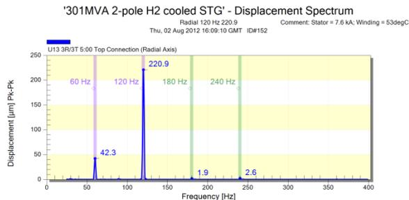
Fig. 1 Displacement spectrum of endwinding vibration accelerometer at 5:00 top connection
