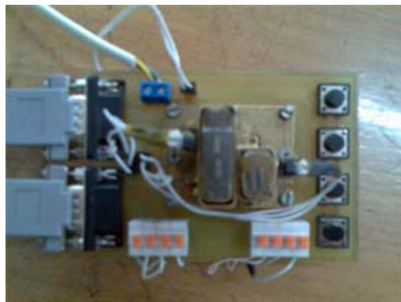
Fig. 4. External view of the actuator of the system of local diagnostics
