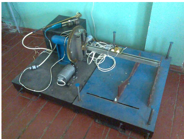
Fig. 3. General view of an industrial model of an automated system of local diagnostics of stator cores
