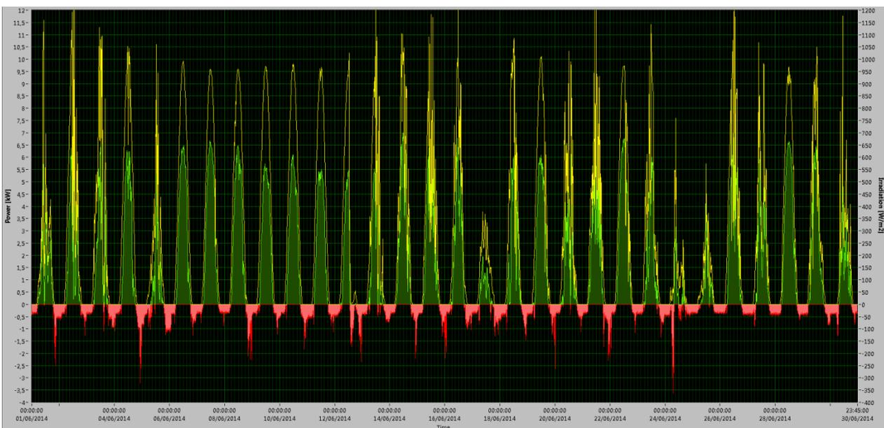
Fig.8. Difference between produced power with PV power plant and the consumed power (monthly measurements)
