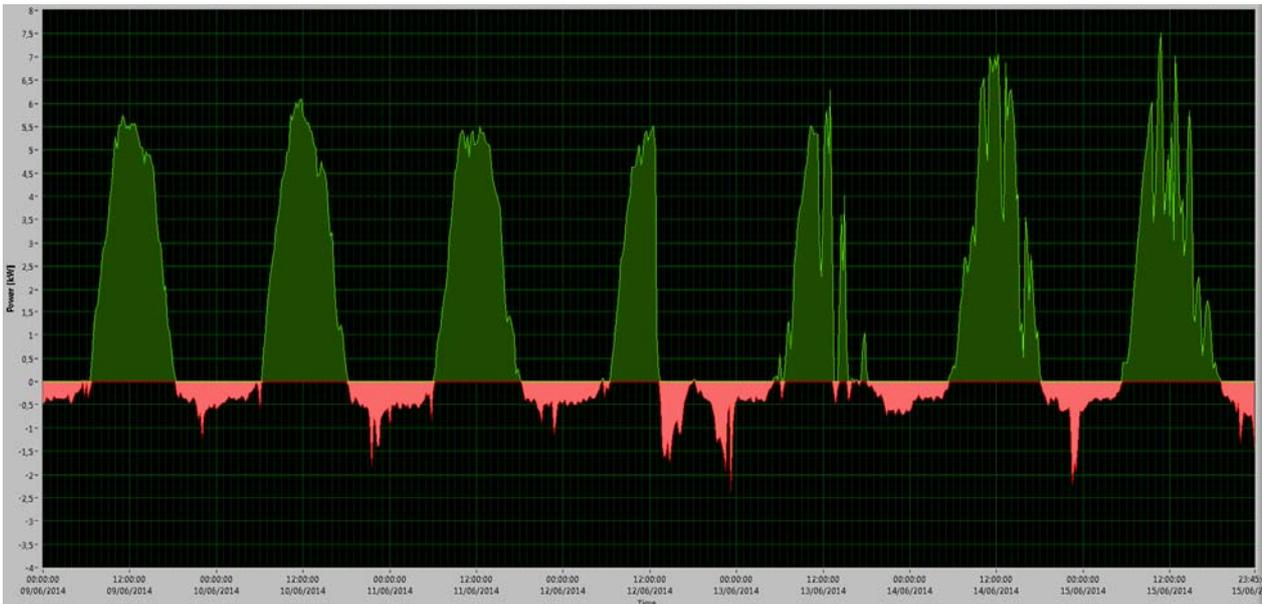
Fig.7. Difference between produced power with PV power plant and the consumed power (weekly measurements)
