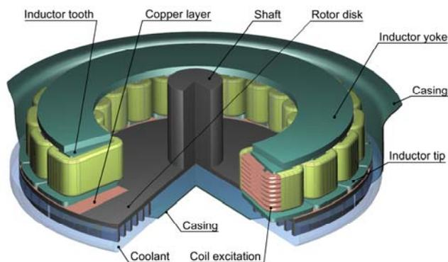
Fig. 1. The sketch of electromagnetic rotating TMEH
