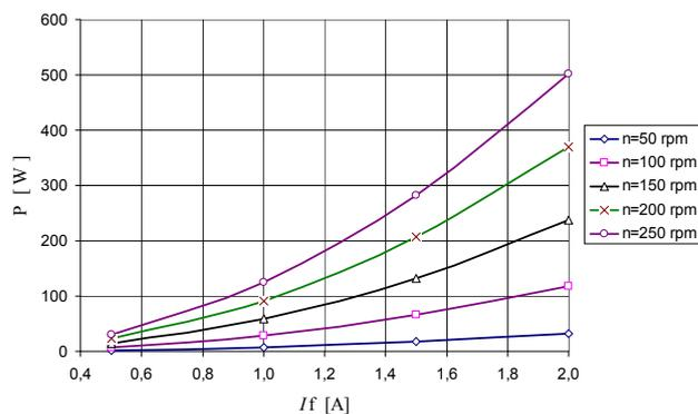
Fig. 8. Dependence of the generated heat power from the excitation current at different rotating speeds in the designed TMEH
