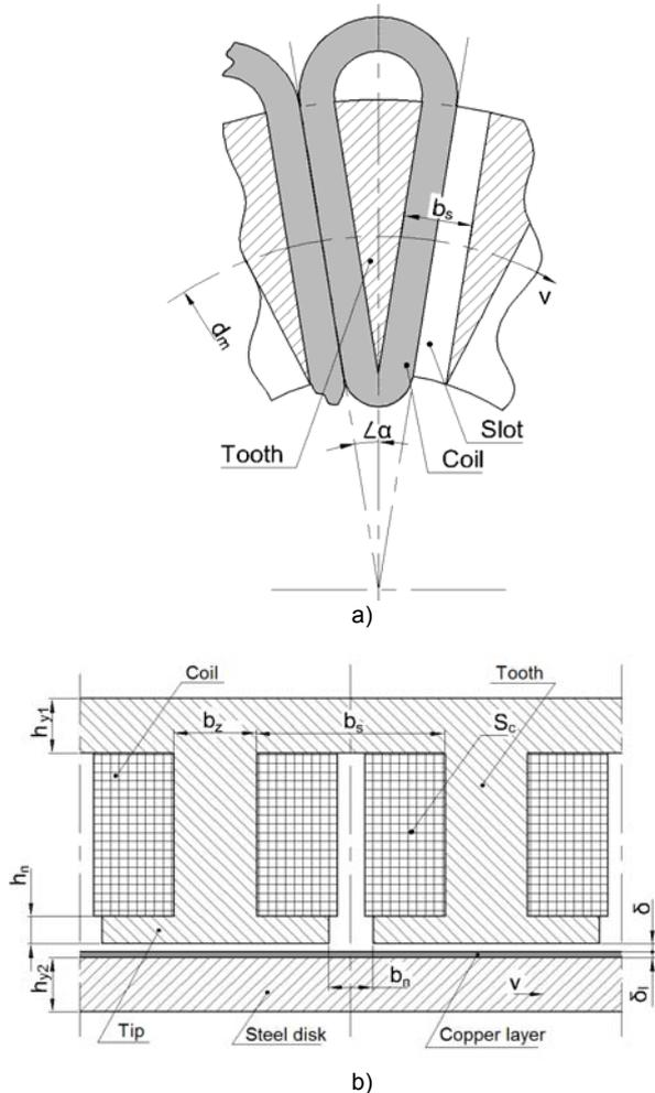
Fig. 5. The sketch of electromagnetic rotating TMEH: a) inductor section in the plane perpendicular to the axis of rotation, b) scan of axial section on the medium diameter of the inductor
