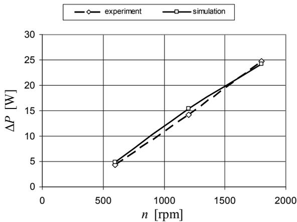
Fig. 4. Dependences of power losses in the aluminum disk rotating in magnetic field of the coil from the rotation frequency for the physical and mathematical experiments
