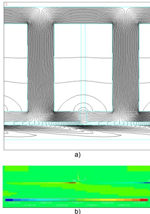
Fig. 6. Results of FEM-analysis of field research in the snippet of the TMEH: a) the distribution of the vector magnetic potential, b) the field of current density vector
