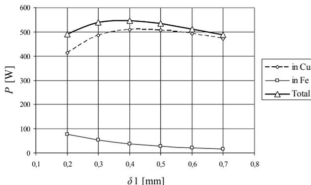
Fig. 7. Dependences of power losses in the layers of rotating disk of the TMEH from the thickness of copper layer on the surface of the steel disk
