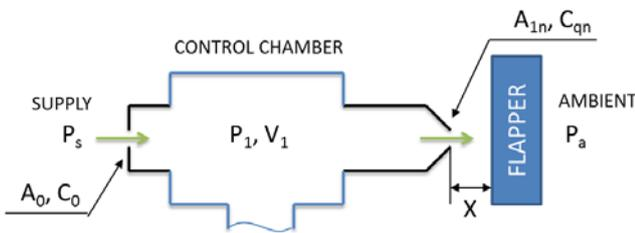
Fig. 13. Schematic of nozzle flapper valve
