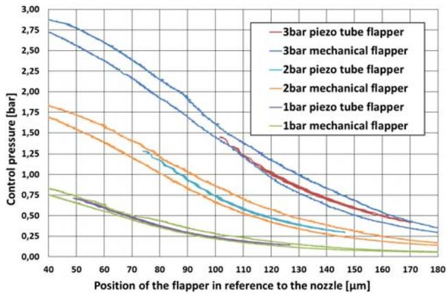
Fig. 9. Comparison of mechanical and piezo driven valve tests results
