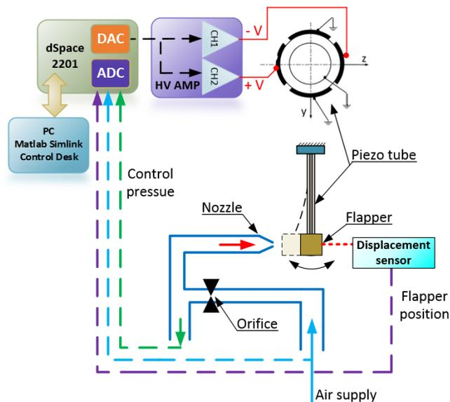
Fig.4. Schematic of designed nozzle flapper valve and test rig
