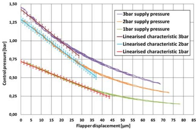
Fig. 8. Pressure regulation of the valve driven by a piezoelectric flapper
