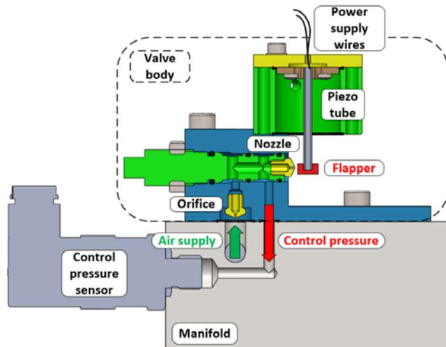
Fig.3. Schematic configuration of the piezo valve system
