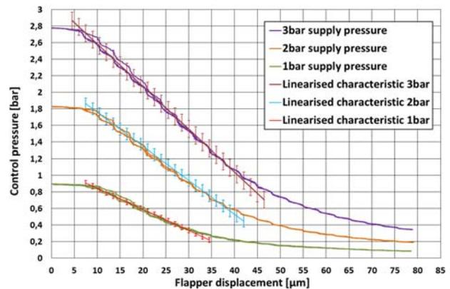
Fig. 11. Pressure regulation of the valve driven by a piezoelectric flapper
