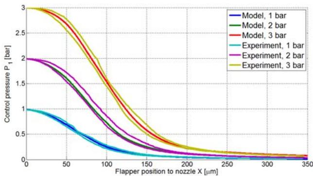
Fig.17. Comparison of mechanical driven valve tests and modelling results for diameter set 1
