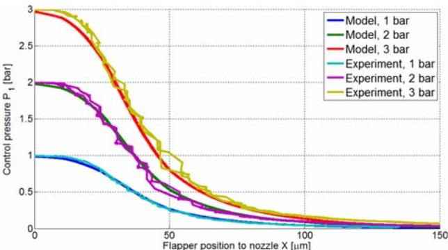
Fig.18. Comparison of mechanical driven valve tests and modelling results for diameter set 2
