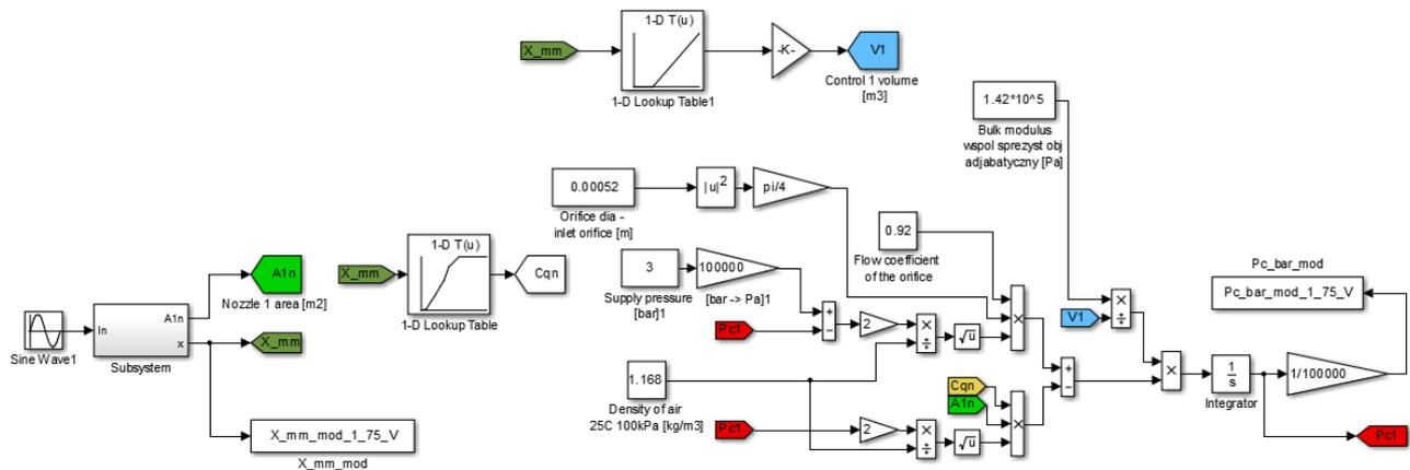
Fig. 14. Matlab-Simulink simplified pneumatic model
