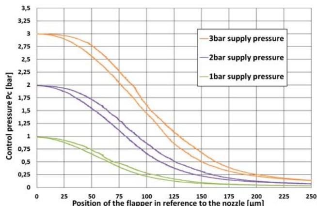
Fig.7. Pressure regulation of the valve driven by a mechanical flapper
