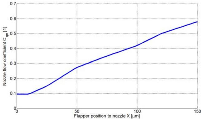
Fig.16. Variation of flow coefficient  $C_{qn}$  for different supply pressure values
