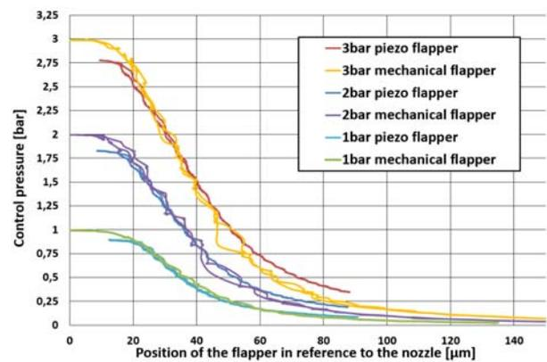
Fig. 12. Comparison of mechanical and piezo driven valve tests results
