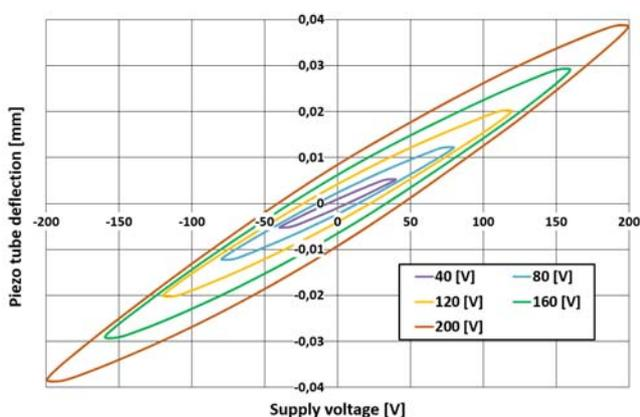
Fig.6. Piezo tube test results
