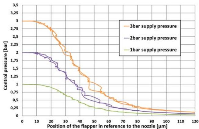
Fig. 10. Pressure regulation of the valve driven by a mechanical flapper
