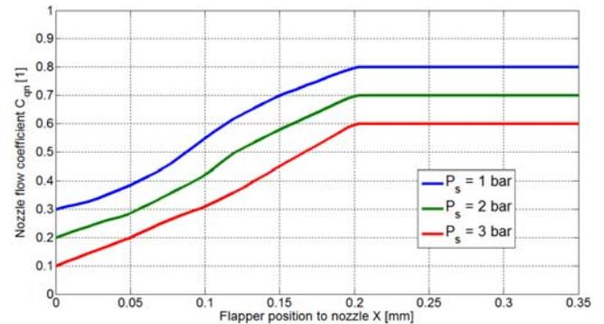
Fig. 15. Variation of flow coefficient  $C_{qn}$  for different supply pressure values
