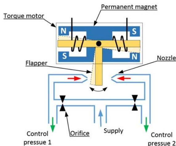
Fig.1. Schematic of a nozzle flapper one-stage servo valve
