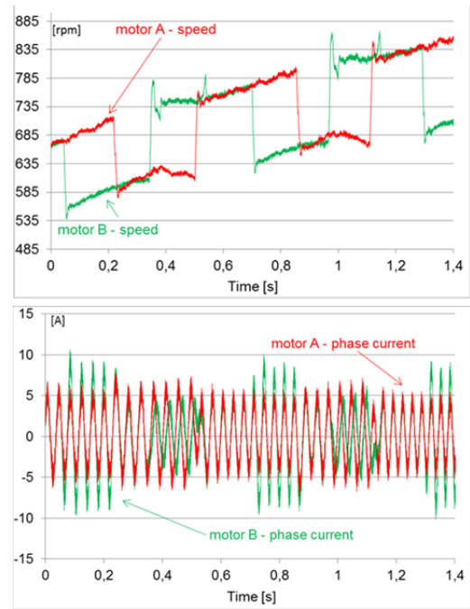
Fig.13. Motor A is the master and motor B is the slave. In this case is used the vector control based on the arithmetic average of the currents measurements of motors A and B, and the measurement of motor A shaft speed
