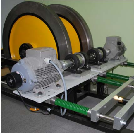
Fig.7. The laboratory stand for modeling transient state of group traction drive
