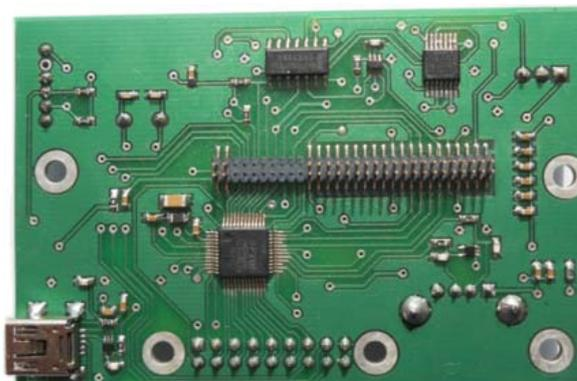
Fig. 3. The bottom layer of the designed USB module
