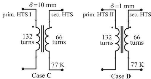
Fig. 3. Diagrams of transformers with windings made of SCS4050 tape
