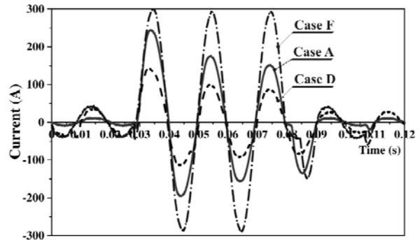
Fig. 13. Time dependent current during current limitation in the primary winding of transformers
