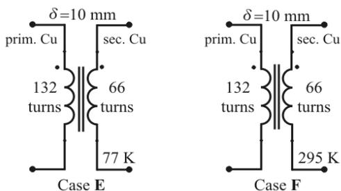
Fig. 4. Diagrams of transformers with windings made of copper wire
