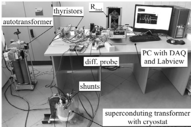
Fig. 9. Experimental setup for short-circuit tests of the transformer
