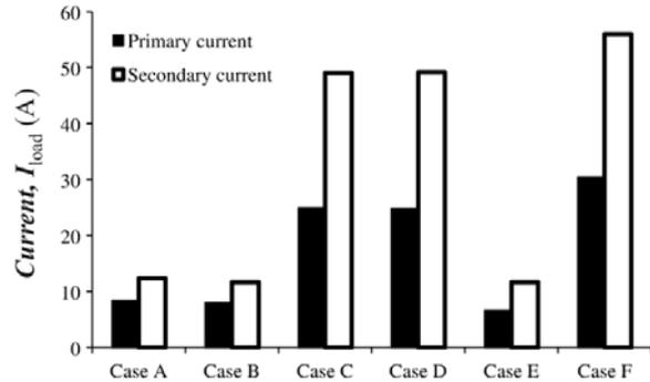
Fig. 11. Comparison of the load current in the transformer windings at  $R_{load} = 8,33 \Omega$
