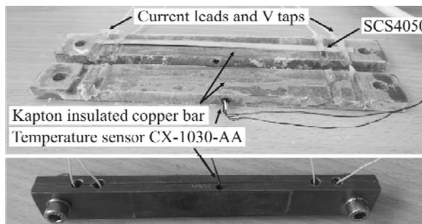
Fig. 7. Experimental setup – HTS tape probe
