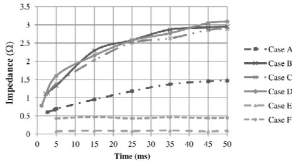
Fig. 14. Comparison of the transformer impedance during the 50 ms fault
