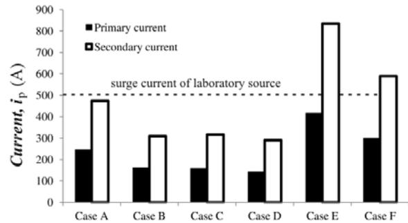
Fig. 12. Comparison of the current's first peak after short in the transformers windings
