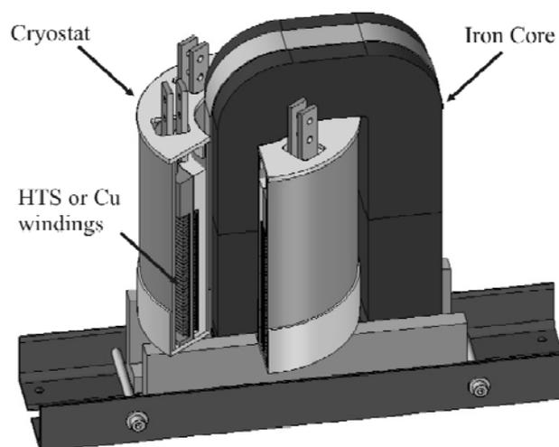
Fig. 1. Model of a 9 kVA superconducting transformer
