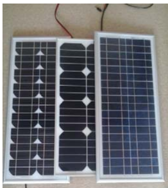
Fig.2. Photovoltaic modules used in current - voltage measurements
