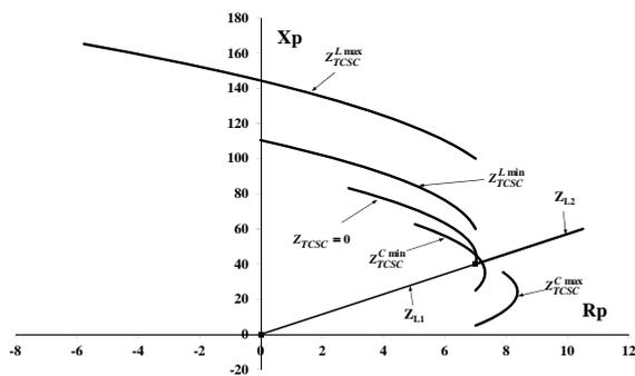
Fig.2 Measurement of impedance by distance protection at the circuit-breaker W1 under metallic short-circuit conditions in transmission line 2 for significant negative angle  $\delta_{13}$
