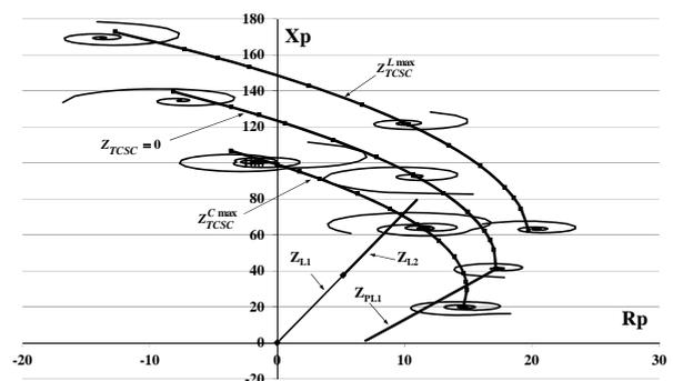
Fig.5 Influence of TCSC controller on measured impedance found in analytical and digital ways, for arc fault and negative angle  $\delta$  under short-circuit on line 2
