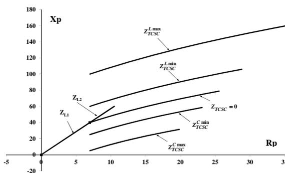
Fig.3 Measurement of impedance by distance protection at the circuit-breaker W1 under metallic short-circuit conditions in transmission line 2 for significant positive angle  $\delta_{13}$
