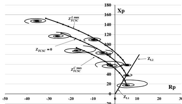
Fig.4 Influence of TCSC controller on measured impedance found in analytical and digital ways, for metallic fault and negative angle  $\delta$  under short-circuit on line 2
