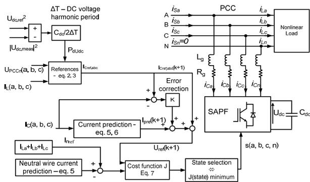
Fig. 4 FS-MPC scheme for SAPF
