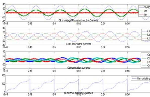
Fig. 5 SAPF with instantaneous power theory based control; Load 2 - operation performance, from the top: phase A grid voltage  $V_a$  and current  $i_{sa}$  (THD=3,9%) and neutral current  $i_{sn}$ , load currents with neutral current, compensation currents, number of switching in SAPF phase A per grid voltage period (20ms)
