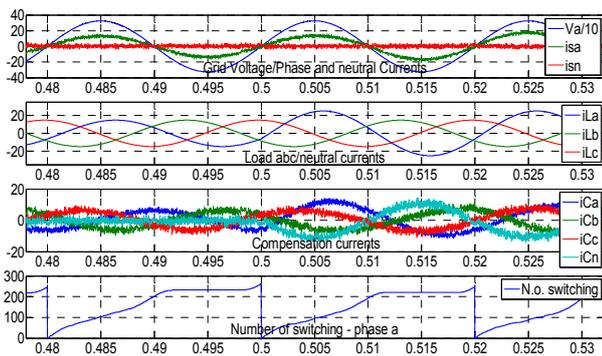
Fig. 7 SAPH with FS-MPC; Load 2 - operation performance, from the top: phase phase A grid voltage  $V_a$  and current  $i_{sa}$  (THD( $i_{sa}$ )=3%) and neutral current  $i_{sn}$ , load currents with neutral current, compensation currents, number of switching in SAPH phase A per grid voltage period (20ms)
