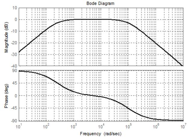
Fig. 6. Bode plot of  $\frac{I_L(s)}{I_L^*(s)}$
