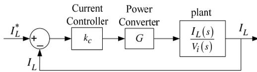
Fig. 4. Inner current loop and plant.
