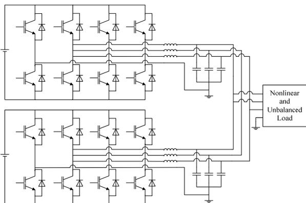
Fig.1. Two parallel four-leg inverters
