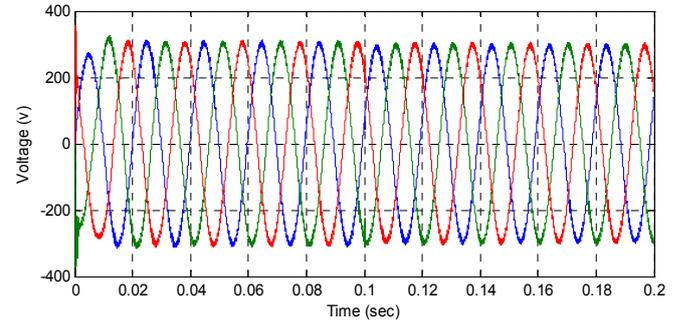
Fig. 12. The output voltage of parallel four-leg inverters.
