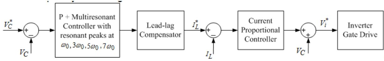
Fig. 10. Block diagram of the voltage control loop based on the proportional-resonant control.
