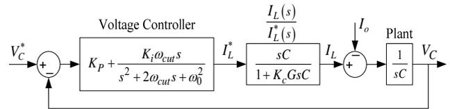
Fig. 7. Proportional-resonant controller for fundamental component.
