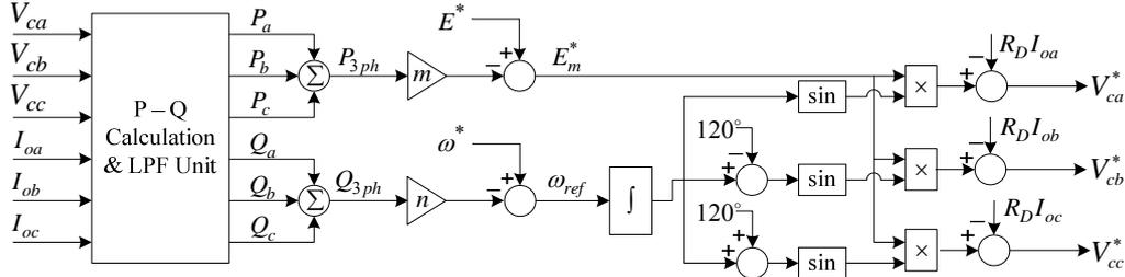
Fig. 11. Block diagram of the voltage control loop based on the proportional-resonant control
