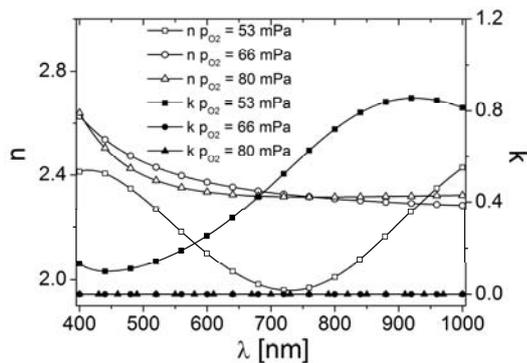
Fig.6. Ti-TiO<sub>2</sub> thin films - n and k versus wavelength for three different oxygen partial pressures
