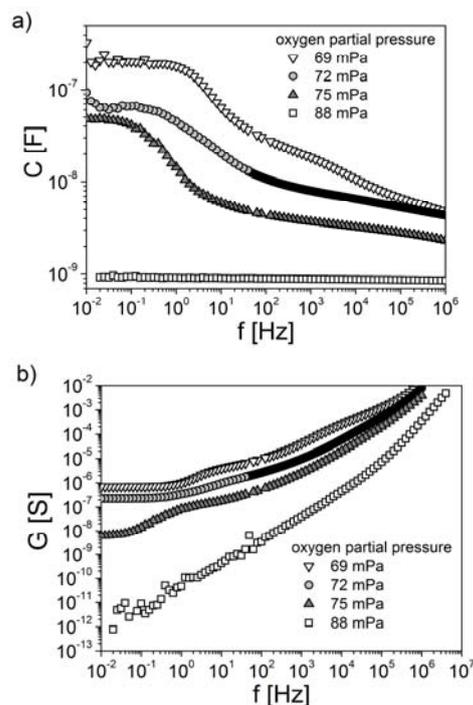
Fig.4. Impedance spectra of the  $Al-(Al_xO_y + Al)-Al$  structure for different oxygen partial pressures: a) capacitance, b) conductance.
