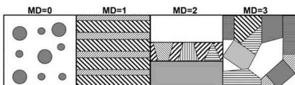
Fig.1 Schematic examples of microstructures for nanostructured coatings
