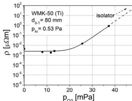
Fig.7. Resistivity versus reactive gas partial pressure of Ti-TiO<sub>2</sub> thin films
