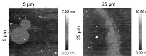
Fig.3. Topographic AFM images of  $Al_xO_y+Al$  composite surface
