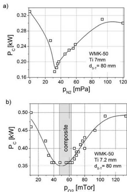
Fig.5. Circulating power  $P_C$  versus reactive gas partial pressure for magnetron sputtering of Ti target: a) sputtering in  $N_2+Ar$  gas mixture b) sputtering in  $O_2+Ar$  gas mixture
