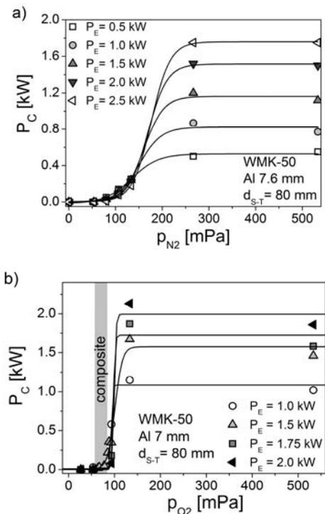
Fig.2. Circulating power  $P_C$  versus reactive gas partial pressure for magnetron sputtering of Al target: a) sputtering in  $N_2+Ar$  gas mixture b) sputtering in  $O_2+Ar$  gas mixture
