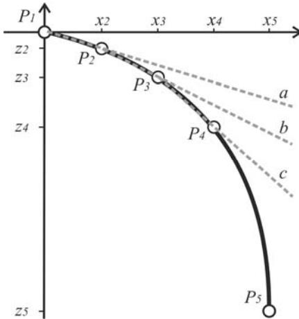
Fig. 7 The illustration of the conditions which allow preserving the monotony of the reflector profile curve
