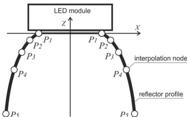
Fig. 1 The reflector model: LED module (light source),  $P_1, P_2, P_3, P_4, P_5$  – interpolation nodes
