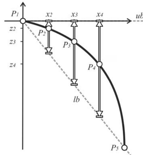
Fig. 2 The reflector profile (version I); the illustration of limiting conditions of the permissible positions of interpolation nodes (points  $P_2, P_3, P_4$ )
