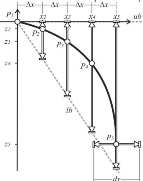
Fig. 3 The reflector profile (version II); the illustration of the limiting conditions of the permissible positions of interpolation nodes (points  $P_1, P_2, P_3, P_4, P_5$ )
