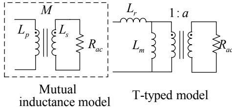
Fig.3. Transformer model of TETS
