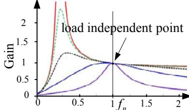
Fig.6. DC characteristic of LLC converter
