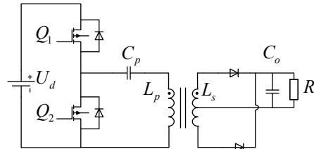
Fig.2. Schematic of proposed half bridge TETS
