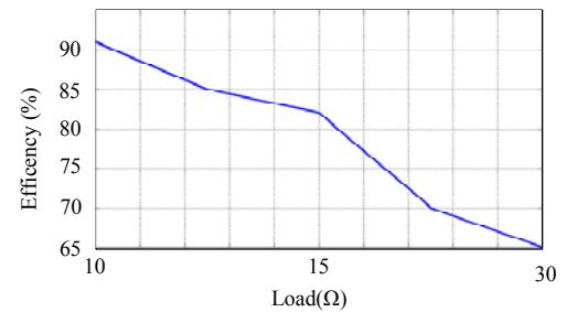
Fig.9. Efficiency of the proposed TETS
