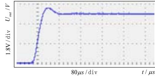
Fig.8. Transient response of LLC resonant TETS
