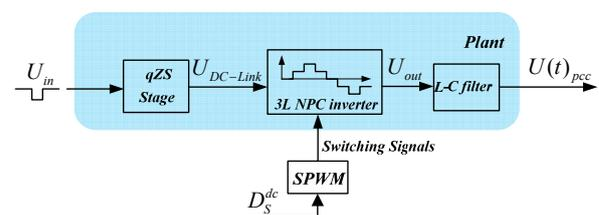
Fig. 2. Open loop block diagram of 3L-NPC qZSI.
