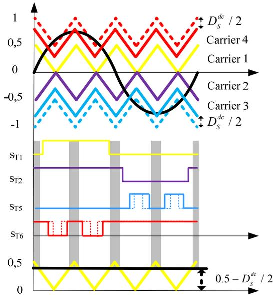
Fig.3. Sketch of the chosen modulation technique.
