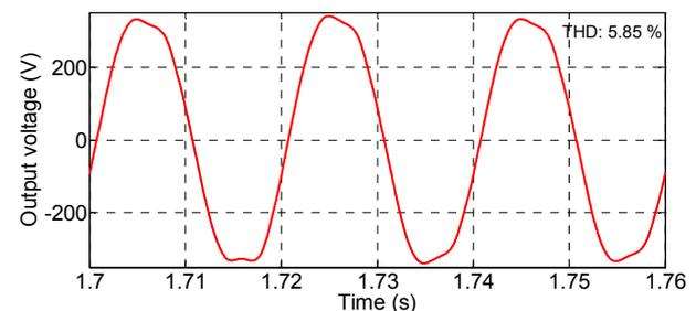
Fig. 16. Output voltage using control system 2.
