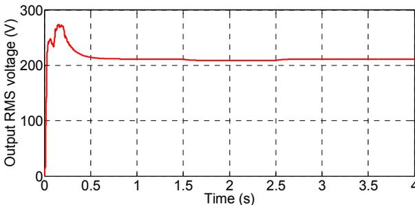
Fig. 11. Output RMS voltage in the 3L-NPC qZSI using control system 2.
