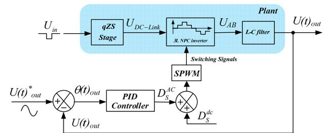
Fig.5. Closed loop block diagram of 3L-NPC qZSI. Proposal 2.
