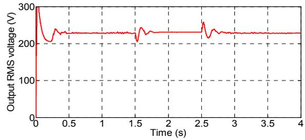
Fig. 13. Output RMS voltage in the 3L-NPC qZSI using control system 3.
