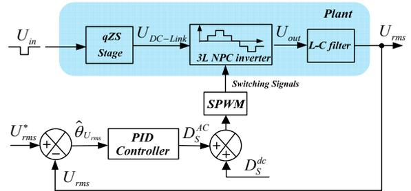
Fig.4. Closed loop block diagram of 3L-NPC qZSI. Proposal 1.
