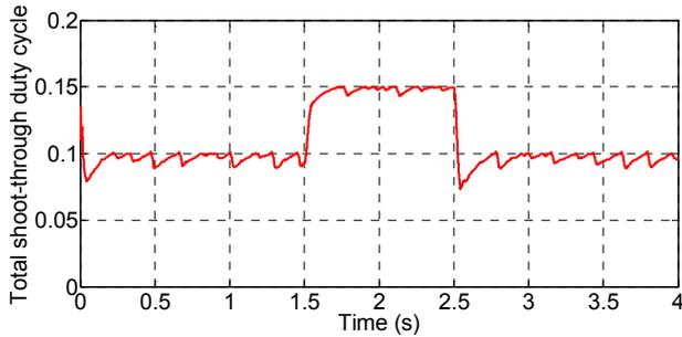
Fig. 10. Total shoot-through duty cycle (constant and variable components) using control system 1.
