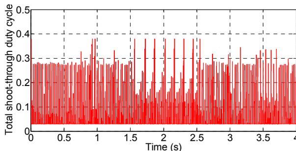
Fig. 12. Total shoot-through duty cycle (constant and variable components) using control system 2.
