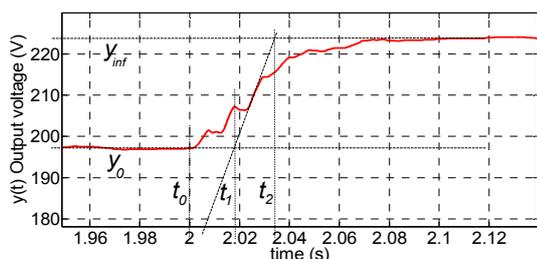
Fig.7. Open loop system response of 3L-NPC qZSI when a step input ( $D^{dc}_s$ ) is applied.
