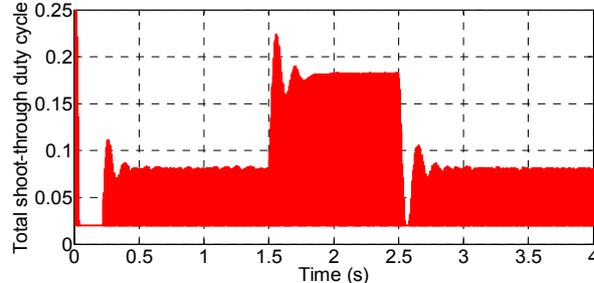
Fig. 14. Total shoot-through duty cycle (constant and variable components) using control system 3.
