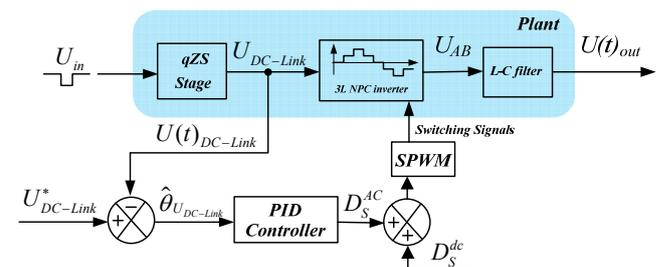
Fig.6. Closed loop block diagram of 3L-NPC qZSI. Proposal 3.
