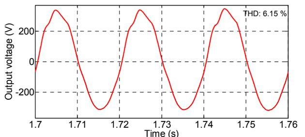
Fig. 17. Output voltage using control system 3.
