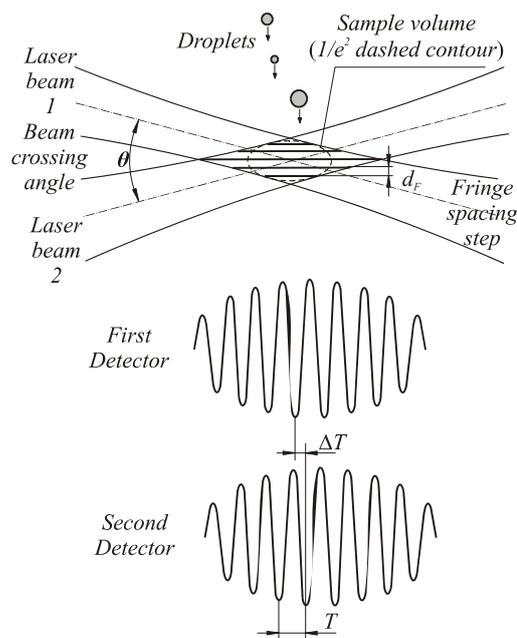
Fig.1. The optical arrangement and measuring principle of PDPA
