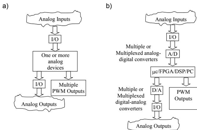
Fig. 1. Comparison of configurable digital and analog signal processing solutions
