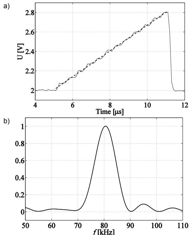
Fig. 9. Signal processing: a) integrator output with its linear approximation; b) Fourier transform of generated sinusoid
