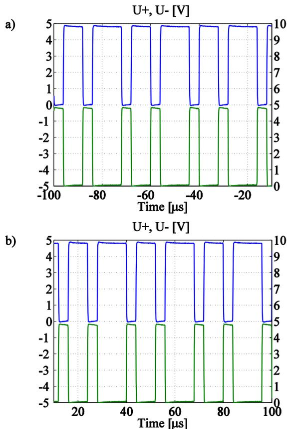
Fig. 10. Comparator output for the user-defined input signal
