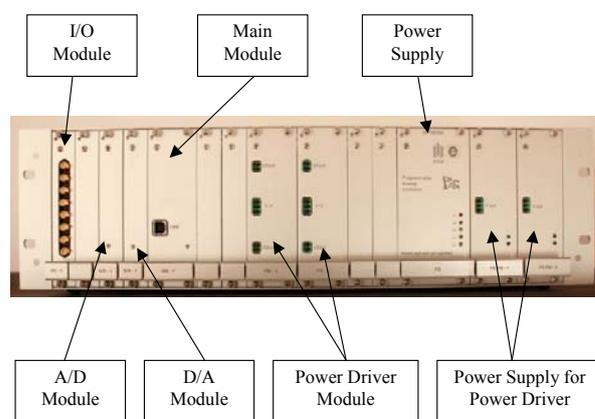
Fig. 2. Programmable Analog Controller in the industrial chassis
