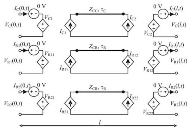
Fig. 3. The complete SPICE model for a three-conductor line [9]
