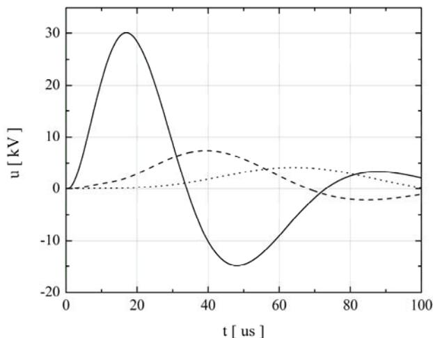
Fig. 9. The courses of voltages for towers from Fig. 7 in splice from rail for the traction system model from Fig. 3
