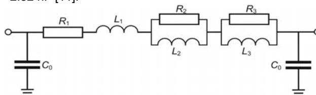
Fig. 2 A frequency- dependent PI section traction system model [5]
