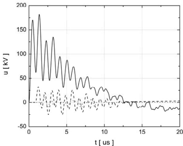
Fig. 7. The courses of voltages for tower in place of lead of impulse wave (the full line) as well as the next one in a distance of 72 (the lined line) and 144m (dotted line) for the traction system model from Fig. 3
