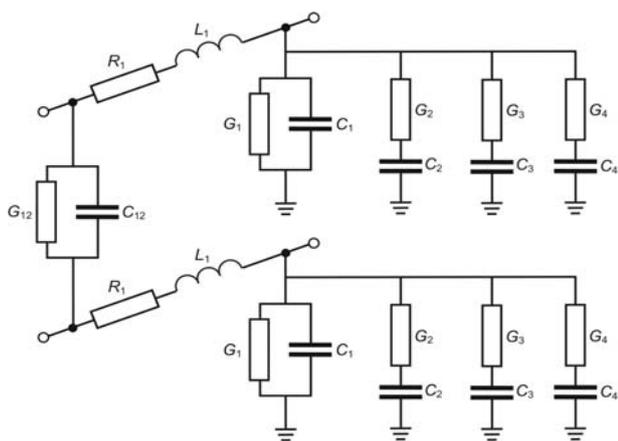
Fig. 4. Scheme of a section of a railway track regarding the influence of the ground [5]
