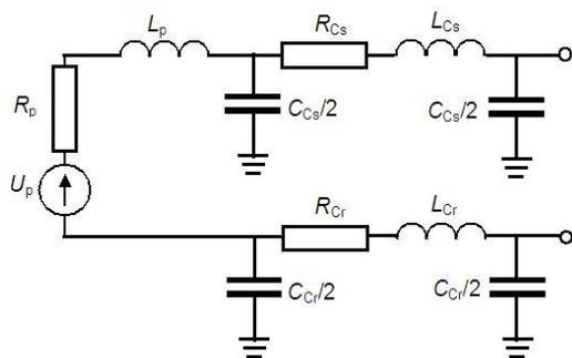
Fig. 5. The scheme of the substations and connections cable [7]
