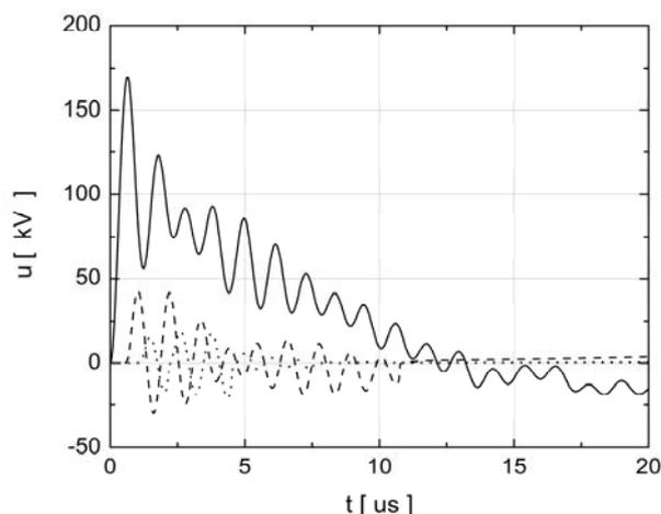
Fig. 6. The courses of voltages for tower in place of lead of impulse wave (the full line) as well as the next one in a distance of 72 ( the lined line) and 144m (dotted line) without the traction system model from Fig. 3
