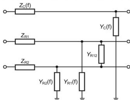
Fig.1. Line rail track impedance and admittance model [5]
