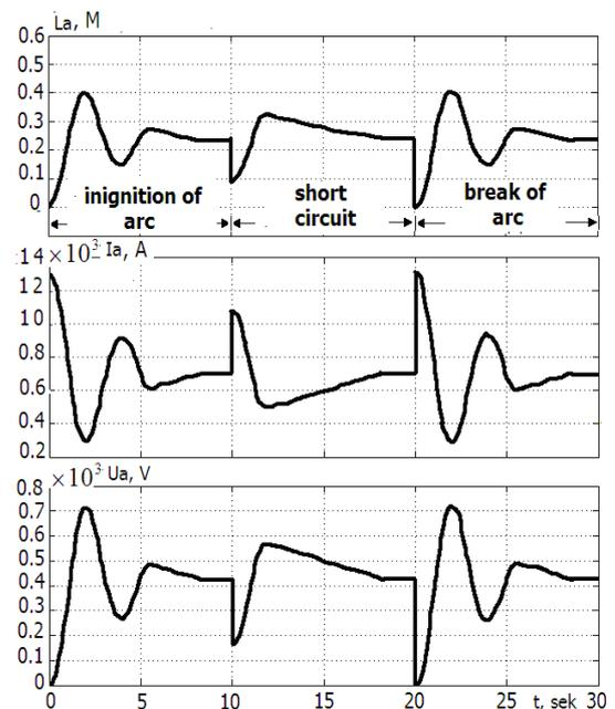
Fig.3. Time dependencies  $l_a(t)$ ,  $I_a(t)$  and  $U_a(t)$  of ARS EM on the base of AFAR-T-12 controller
