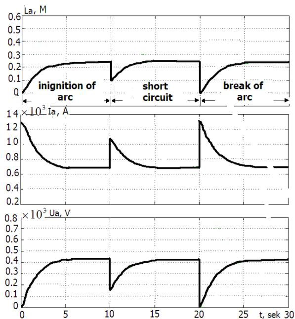
Fig.4. Time dependencies  $I_a(t)$ ,  $I_a(t)$  and  $U_a(t)$  ARS EM with a neuro-controller
