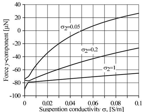
Fig.4. Dependence of the x-component of the force  $\mathbf{F}$  acting on particle from fluid conductivity. Conductivity of the particle in S/m is a parameter..
