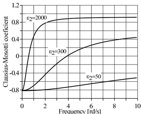
Fig.2. Dependence of the real part of the Clausius-Mosotti coefficient from frequency. Relative permittivity of particle is as parameter.
