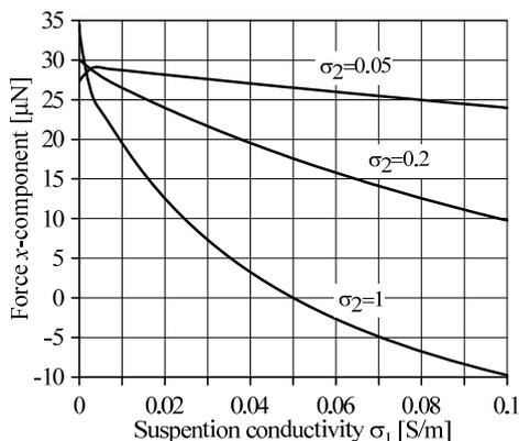
Fig.3. Dependence of the x-component of the force  $\mathbf{F}$  acting on particle from fluid conductivity. Conductivity of the particle in S/m is a parameter.
