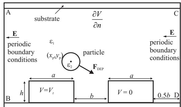
Fig.1. Single electrode arrangement in dielectrophoretic trap.
