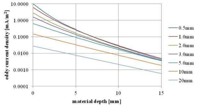
Fig.2. Dependences of eddy current density in absolute values on the material depth for different adjustments of lift-off,  $r_c = 2$  mm
