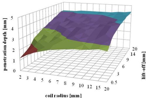
Fig.6. Penetration depth as function of coil radius and lift-off
