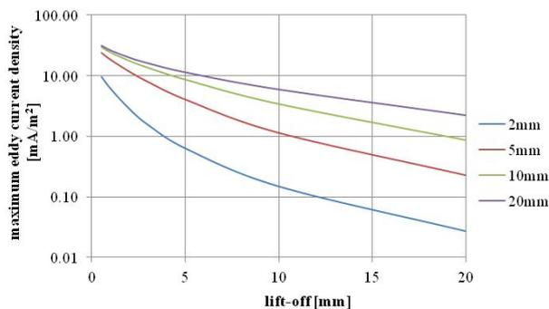
Fig.7. Dependences of maximum eddy current density in absolute values on the lift-off for the coil with various radiuses
