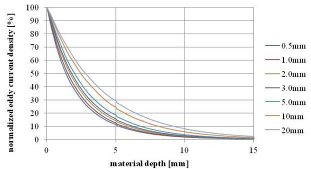
Fig.4. Dependences of eddy current density in relative values on the material depth for different adjustments of lift-off,  $r_c = 5$  mm
