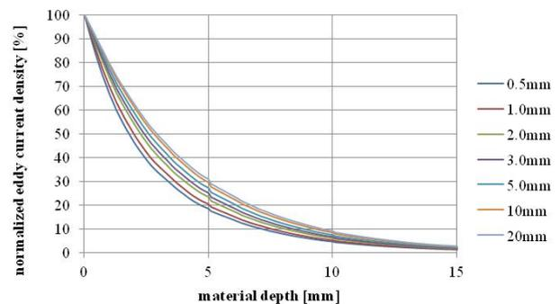
Fig.5. Dependences of eddy current density in relative values on the material depth for different adjustments of lift-off,  $r_c = 20$  mm
