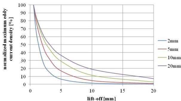
Fig.8. Dependences of maximum eddy current density in relative values on the lift-off for the coil with various radiuses
