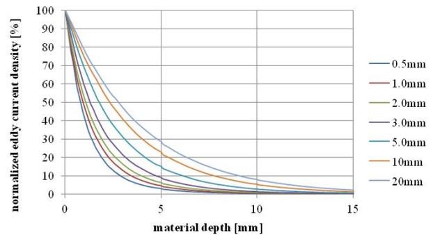
Fig.3. Dependences of eddy current density in relative values on the material depth for different adjustments of lift-off,  $r_c = 2$  mm
