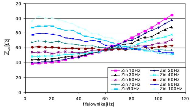
Fig. 8 Module of input impedance of a drive system in the function of inverter frequency  $f_{fal}$ , for selected frequencies with constant depth of modulation  $M_{mod}=0,6$
