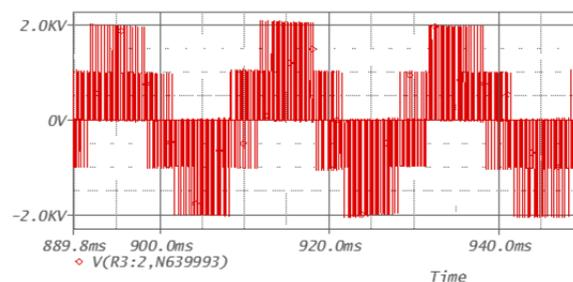
Fig.4 Exemplary runs of phase voltage with a 3-phase supply of load of type RL by a voltage inverter with PWM modulation
