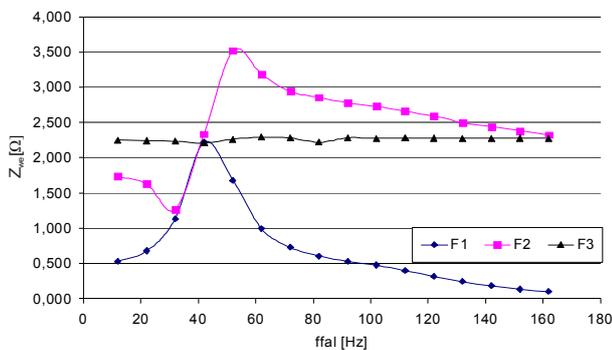
Fig. 10 Results of determination of input impedance module in the function of frequency of one drive group for three versions of an input filter F1 ( $L_f = 8,7$  mH,  $C_f = 1$  mF); F2 ( $L_f = 16$  mH,  $C_f = 1$  mF); F3 ( $L_f = 8,7$  mH;  $C_f = 6,5$  mF)
