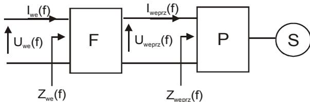
Fig. 1 Schematic diagram for identification of current and voltage measurements points necessary for determination of input impedance:-F- converter input filter; P-converter; S-traction motor
