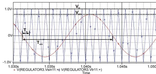
Fig. 2 Runs of signals compared to the generation of runs which control inverter branches, where:  $V_{sin}$ - an amplitude of sinusoidal signal,  $V_{tr}$  - an amplitude of triangular signal,  $T_{sin}$  - a period of sinusoidal signal,  $T_{tr}$  - a period of triangular signal
