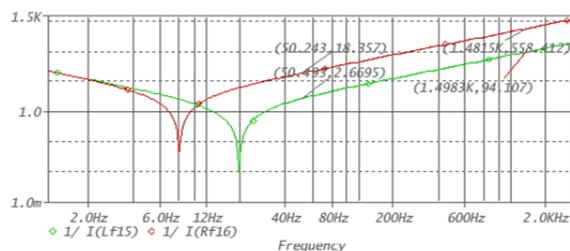
Fig. 12. Characteristics of impedance module of exemplary input filters allowing for the fulfilment of the norm PN-EN 50388 [13] for multiple-operation of a 4-motor vehicle with accordance to the a) effective version ( $1/(L_f15)$   $L_f = 10$ mH), b) previous version ( $1/(L_f16)$   $L_f = 60$ mH)
