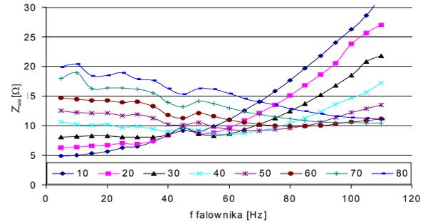
Fig. 7 Runs of system input impedance module for selected frequencies in the function of inverter operation frequency  $f_{fal}$ .
