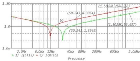
Fig. 13. Characteristics of impedance module of exemplary input filters allowing for the fulfilment of the norm PN-EN 50388 [13] for individual traction of a 4-motor vehicle with accordance to the a) effective version ( $1/I(Lf15)$   $L_f = 6mH$ ), b) previous version ( $1/I(Lf16)$   $L_f = 28mH$ )
