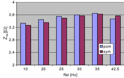
Fig. 6 Comparison of the results of impedance module determination by computer simulation (sym) with the results of laboratory measurements (pom) for various frequencies of converter operation ( $f_{fal}$ ) with inductance of input filter  $L_{F1} = 1,8$ mH a) impedance for harmonic 41 Hz b) impedance for harmonics 46 Hz
