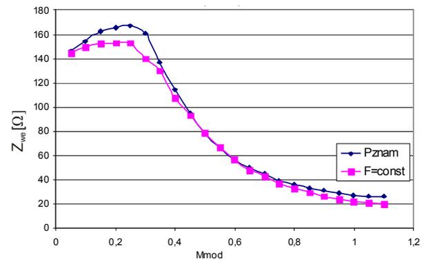
Fig. 9 Module of input impedance of a drive system in the function of modulation depth for the frequency of 50 Hz, where:  $P_{znam}$  - frequency of an inverter that changes fluently together with modulation depth  $F_{const}$  - constant inverter frequency
