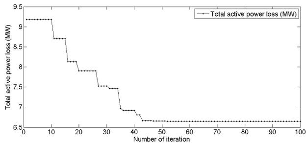
Fig.5. Variation of total active power loss against iteration for proposed approach ( $P_{base} = 100MW$ )
