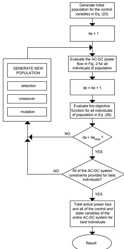
Fig.3. The proposed flow chart for ORPF in multi-terminal ac-dc system by GA
