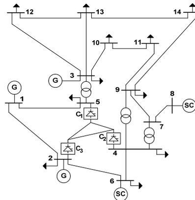
Fig.4. The modified IEEE 14-bus ac-dc test system
