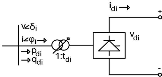
Fig.1. Equivalent representation of a mono-polar converter station
