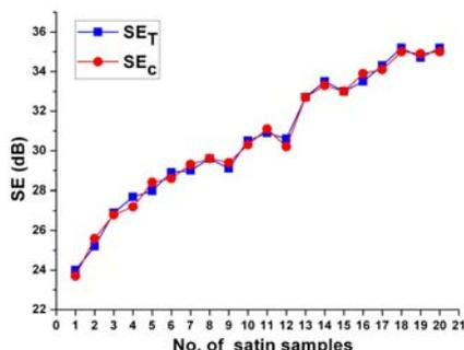
Fig.5. Comparisons between the SE testing results and the SE computation results of the satin weave fabric
