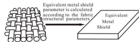
Fig.1. Equivalent metal shield
