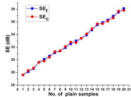
Fig.3. Comparisons between the SE testing results and the SE computation results of the plain weave fabric
