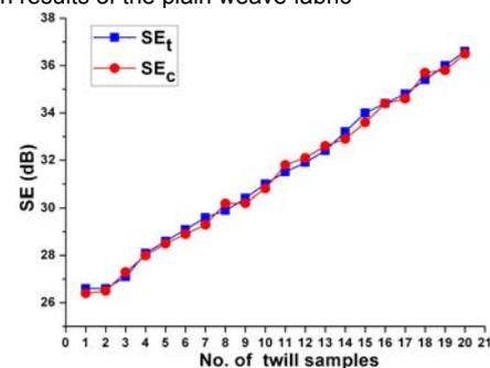
Fig.4. Comparisons between the SE testing results and the SE computation results of the twill weave fabric
