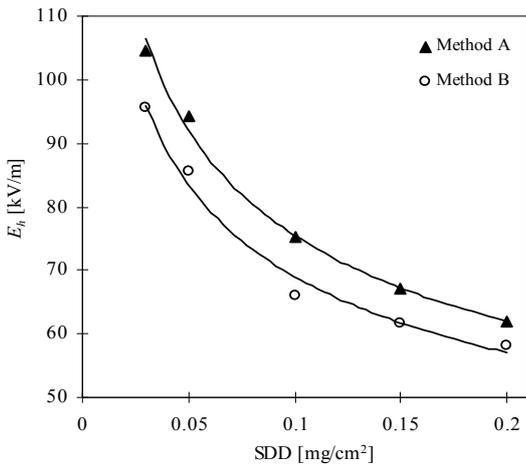
(b) AC flashover voltage gradient of type B insulator string
