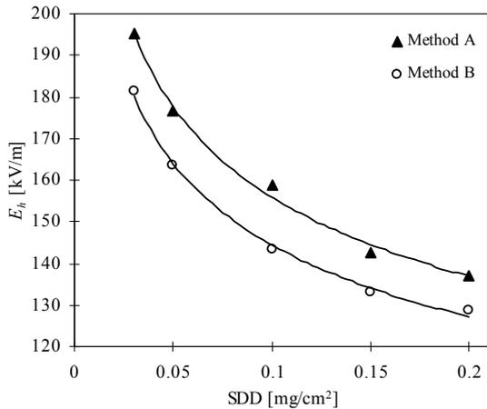
(a) AC flashover voltage gradient of type A insulator
