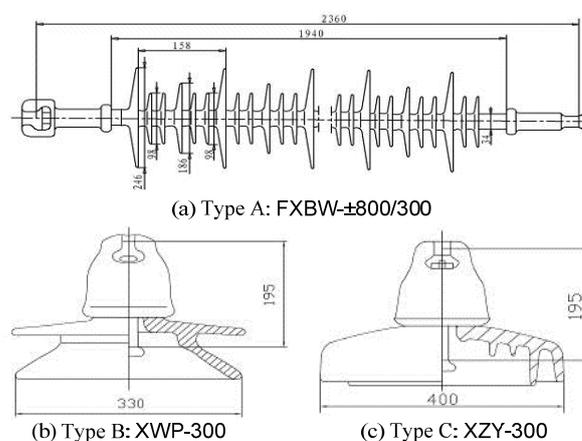
Fig.1. Configuration of the tested insulators
