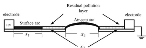
$x_1$ : length of surface arc,  $x_2$ : length of air-gap arc,  $x_3$ : length of residual pollution layer
