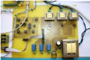
a) The voltage detection card Fig. 4. The measurement cards
