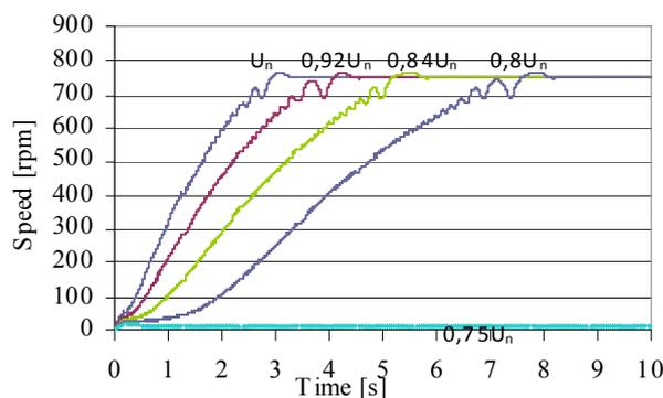
Fig. 5 Transient of rotational speed during motor start for different voltage drops in the supply network.
