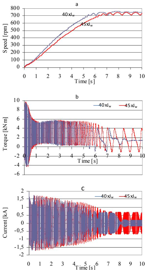
Fig. 6 Transients of rotational speed (a), electromagnetic torque (b) and phase current (c) during the start of the motor with different values of the drivetrain moment of inertia.
