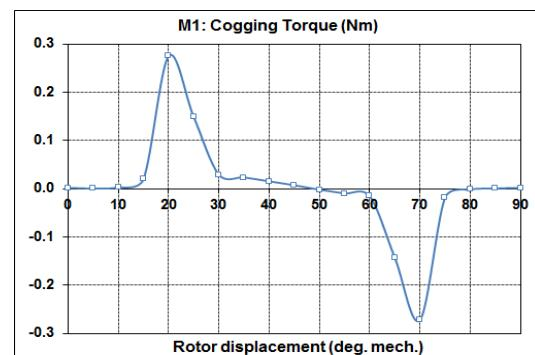
Fig. 7. Cogging torque of the generic model of BLDCPM motor-M1
