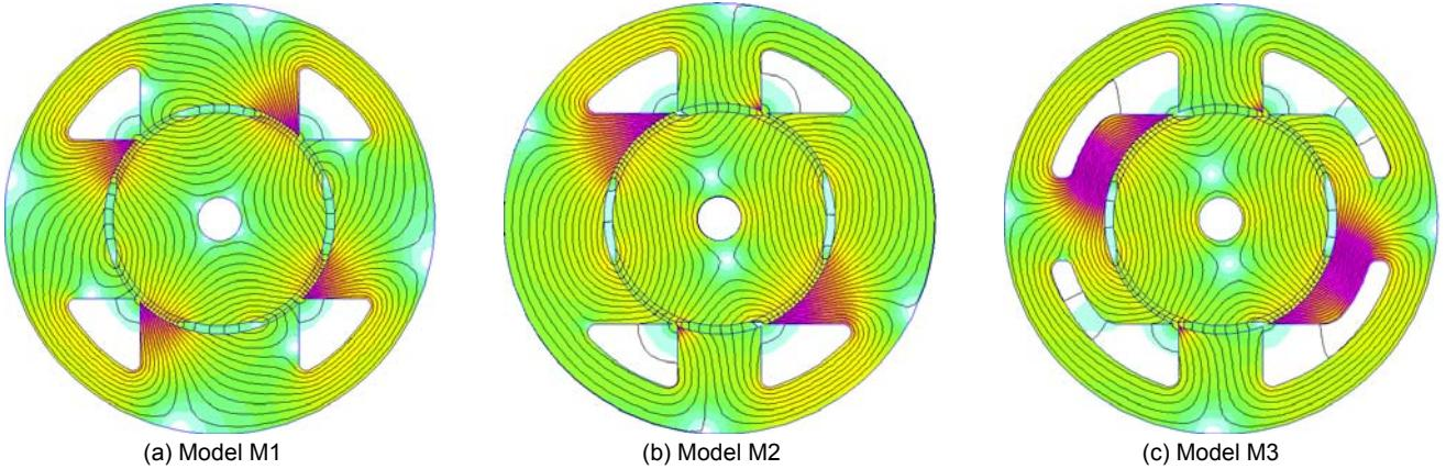
Fig. 5. Field distribution at rated current and  $45^\circ$  rotor position in the derived models of BLDCPM motor M1, M2 and M3
