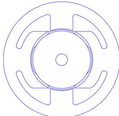
Fig. 3. Shaping the stator poles of BLDCPM motor – M3
