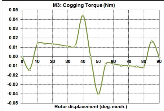
Fig. 9. Cogging torque of M3 – pole ratio 1:3 and shaped poles
