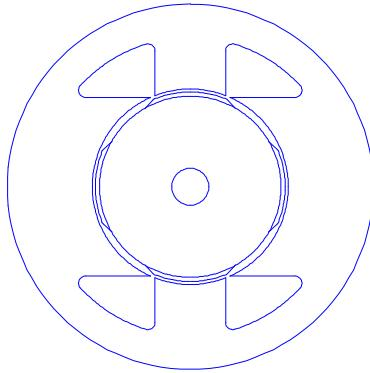
Fig. 2. Design development of BLDCPM motor: pole ratio 1:3 – M2
