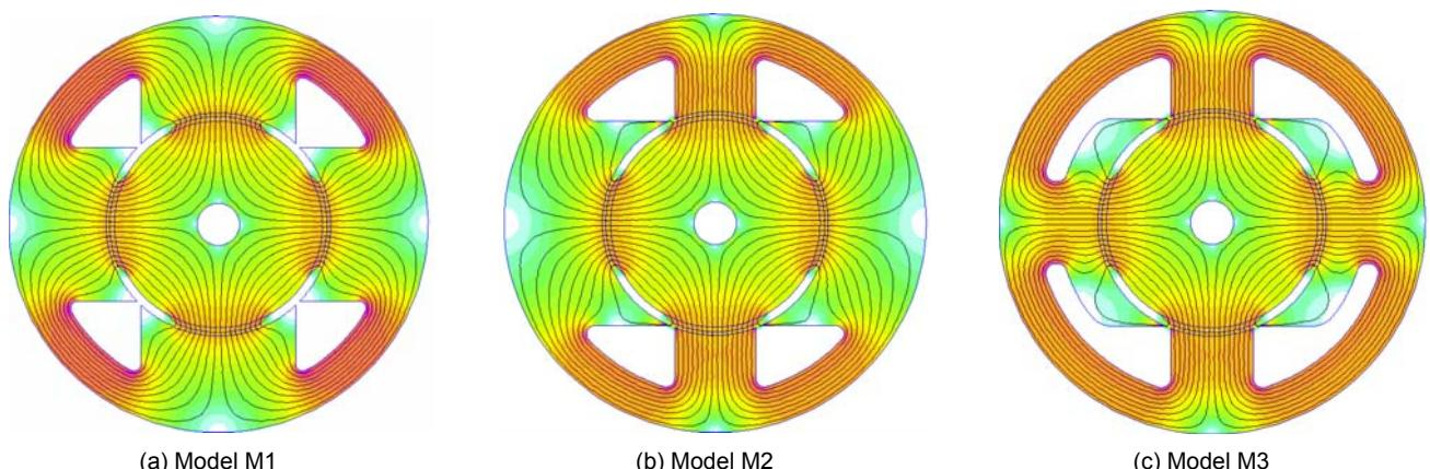
Fig. 4. Field distribution in unexcited BLDCPM motor and  $0^\circ$  rotor position in the derived models M1, M2 and M3
