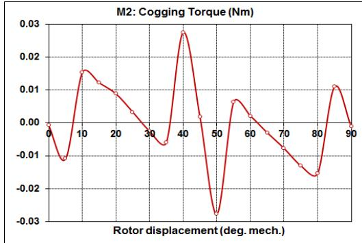
Fig. 8. Cogging torque of the model M2 – pole ratio 1:3
