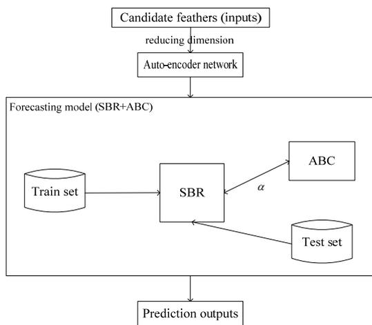
Fig 1. Structure of the proposed wind power forecast strategy
