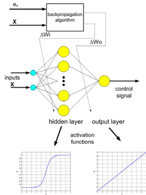
Fig. 2. Structure of the neural network trained on-line
