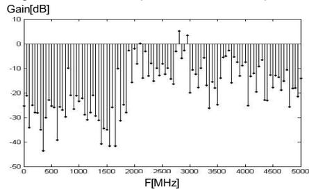
b) The gain measured at probe 6 relative to probe 4
