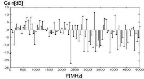
Fig.6. Electric field signal's relative gain measured by the probes on the front and the back of insulators
