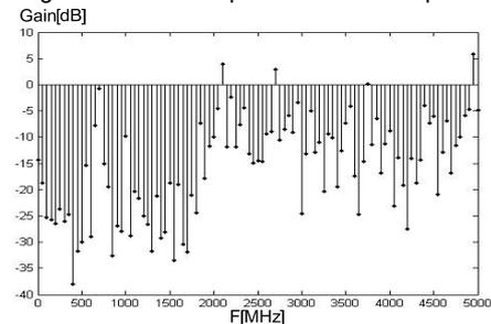
Fig.7. Electric field signal gain of the leaked electromagnetic wave
