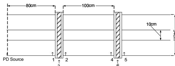
Fig.4. Position of excitation source and probes
