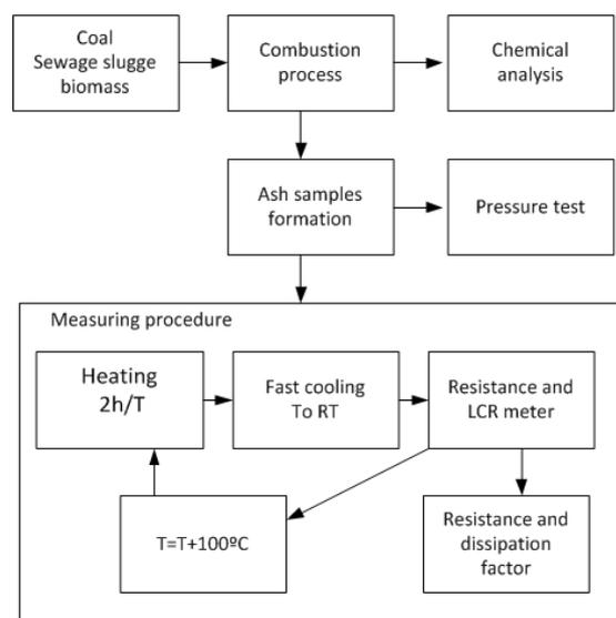
Fig.1. The testing procedure.
