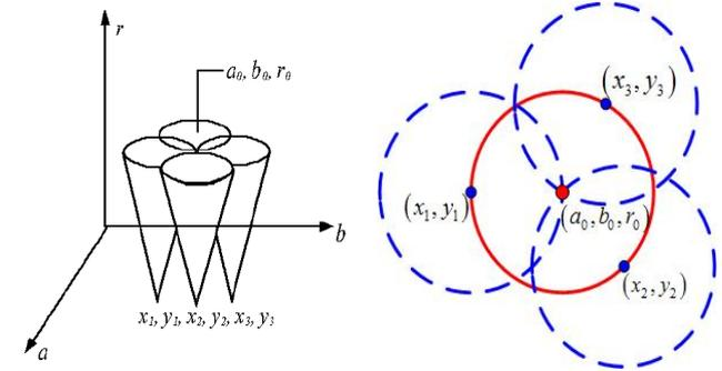
Fig.3. Hough transform and circle detection
