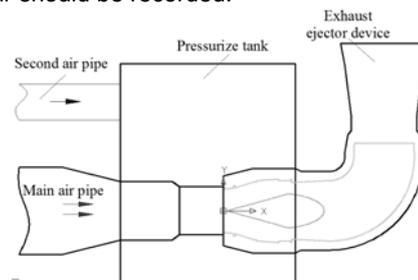
Fig.6. The arrangement of experimental facilities
