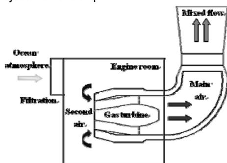
Fig.1. Arrangement plan of the exhaust ejector
