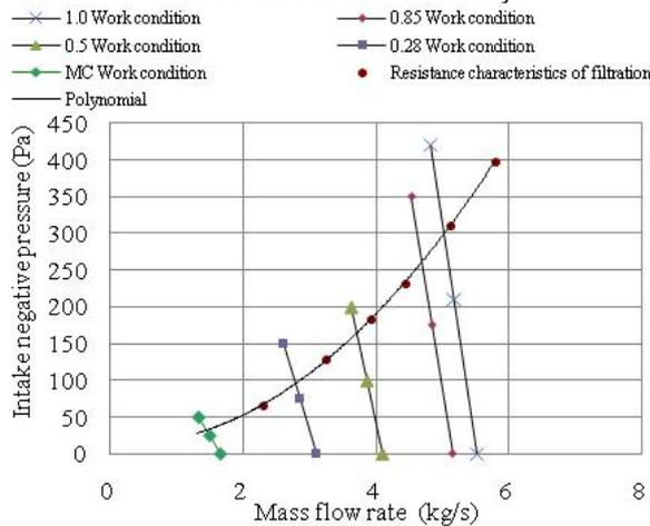
Fig.4. The curve about flow rate and negative pressure of the second air
