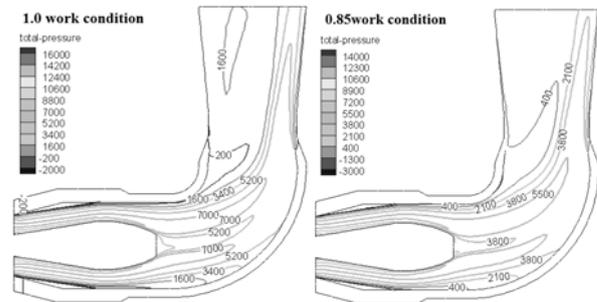
Fig.5. Pressure contours distribution of vertical section
