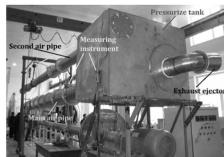
Fig.7. The local arrangement of experimental facilities
