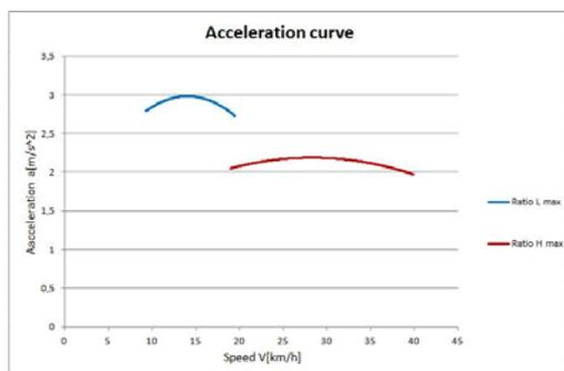
Fig.6. UTV vehicle acceleration curve - combustion engine
