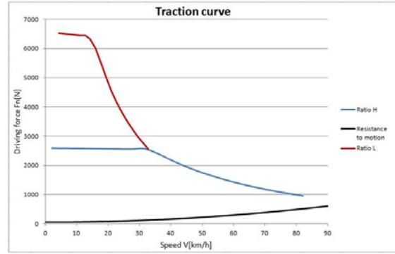
Fig.3. UTV vehicle traction curve - electric motor
