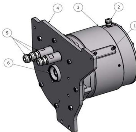
Fig.2. Conceptual model of electric engine with permanent magnets
