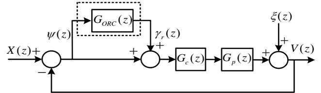
Fig. 3. General block diagram of control scheme
