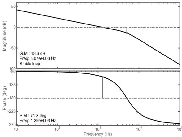
Fig. 4. Bode diagram of the output current transfer function
