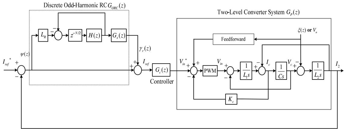
Fig. 2. Overall block diagram of the ORC system of the two-level converter incorporated in the basic classical controller
