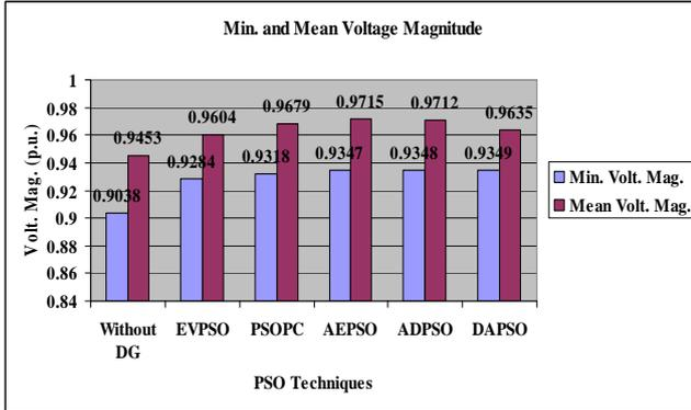
Fig. 3. Min. and mean voltage values for different PSO techniques in Case-I
