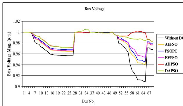
Fig. 7. IEEE 69-bus radial distribution system bus voltage for PSO techniques
