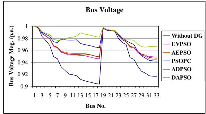
Fig. 4. IEEE 33-bus distribution system voltage profile in Case-II
