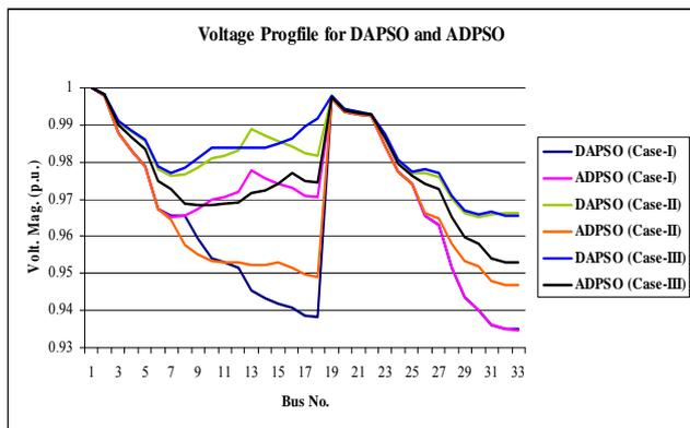
Fig. 6. IEEE 33-bus radial distribution system bus voltage for DAPSO and ADPSO in Case-I, Case-II and Case-III
