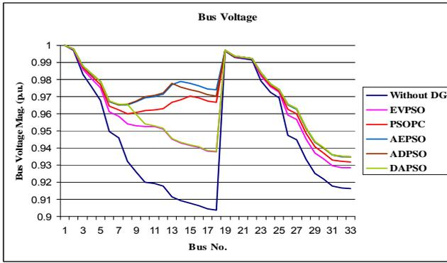
Fig. 2. IEEE 33-bus radial distribution system bus voltage in Case-I
