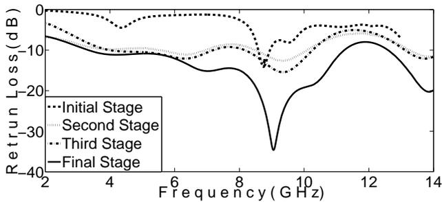
Fig. 2. Effect of stages on Return Loss.
