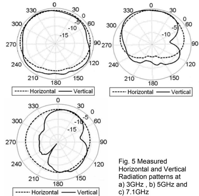
Fig. 5 Measured Horizontal and Vertical Radiation patterns at a) 3GHz, b) 5GHz and c) 7.1GHz
