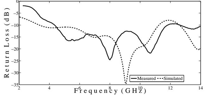
Fig. 4. Simulated and measured results of final stage
