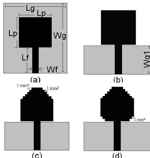
Fig. 1. Geometrical structure of a)First Stage, b)Second Stage, c)Third Stage d)Fourth Stage.
