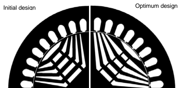
Figure.9. Configurations of optimized and initial design model for rotor design
