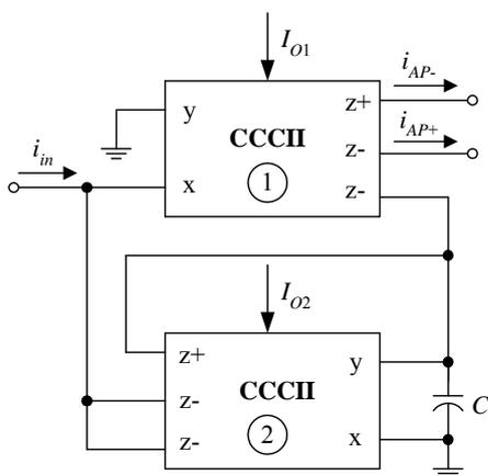
Fig.2. Proposed electronically tunable current-mode first-order allpass filter.
