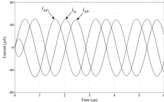
Fig.6 Time-domain responses of the proposed AP filter for input frequency 612 kHz.
