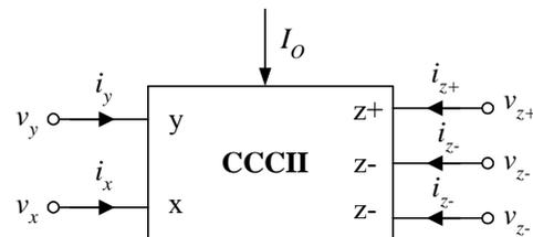
Fig.1. Circuit symbol of the CCCII.
