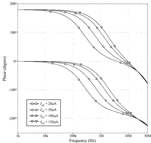
Fig.5. Electronically tunable phase response of the proposed AP filters.
