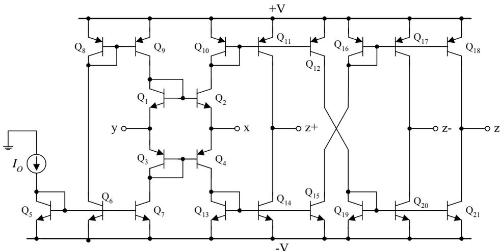
Fig.3. Bipolar technology implementation of the CCCII.
