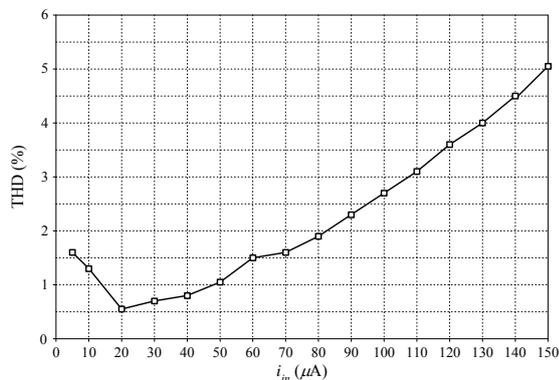
Fig.7 THD variations with respect to peak value of applied sinusoidal input current.
