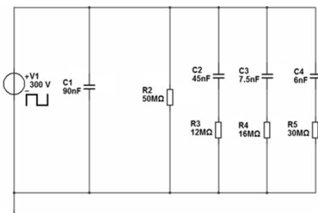
Fig.3. Principle circuit for simulating relaxation currents
