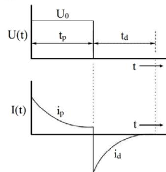
Fig.2. Principle waveform of relaxation currents [4]
