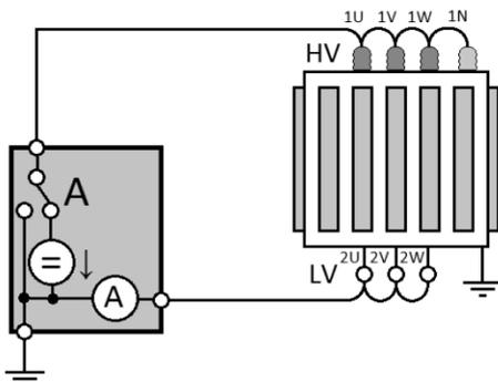
Fig.1. Simply PDC measurement system
