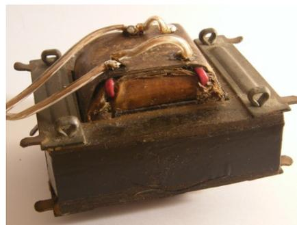
Fig.4. Measured transformer TESLA 230V~24V
