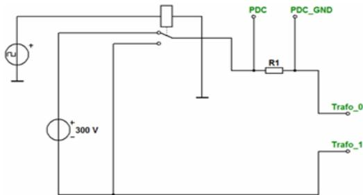
Fig.6. Principle circuit for measuring relaxation currents
