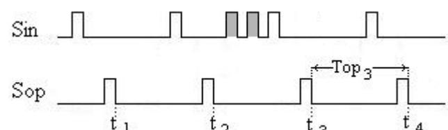
Fig. 4 Black pulses are eliminated;  $T_{op3}$  is decreased for two  $t_c$
