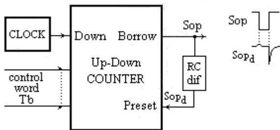
Fig. 2 The principal scheme of the programmable period generator
