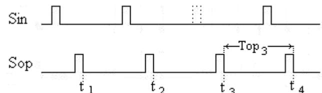
Fig. 3 The lost pulse is recovered;  $T_{op3}$  is increased for  $t_c$
