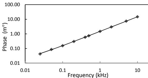
Fig. 5. Frequency dependence on the phase value of complex voltage ratio
