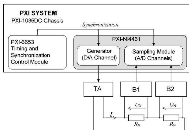
Fig. 1. Simplified diagram of the system for resistor calibration
