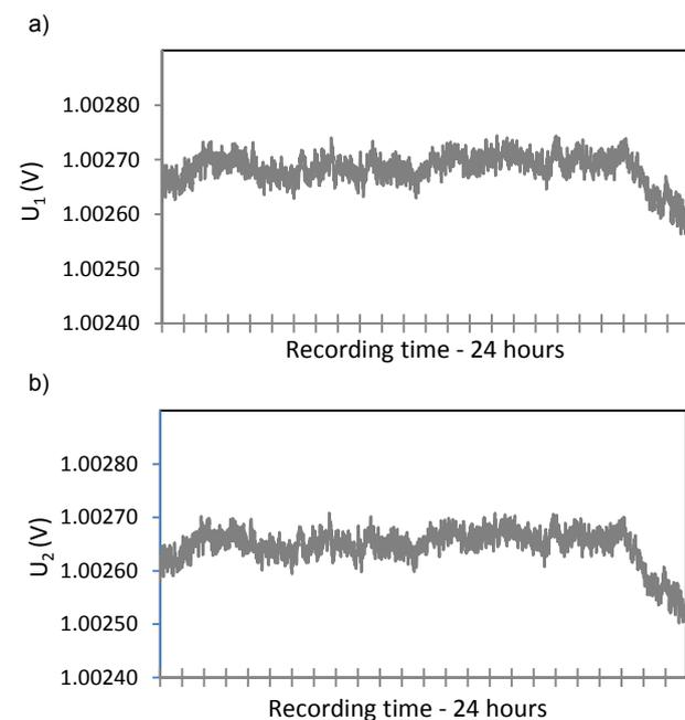
Fig. 2. Voltages measured by: a) channel 1, b) channel 2 of the digitizer; the measuring range is  $\pm 1$  V
