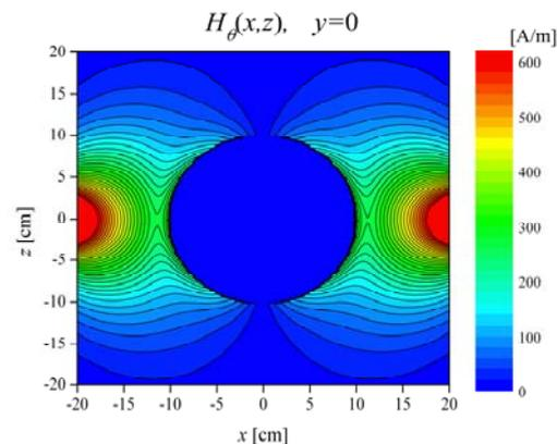
Fig. 8. Computed distribution for the zenith component of the magnetic field intensity
