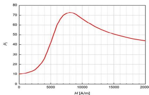
Fig. 4.  $\mu(H)$  dependence (steel ST35)
