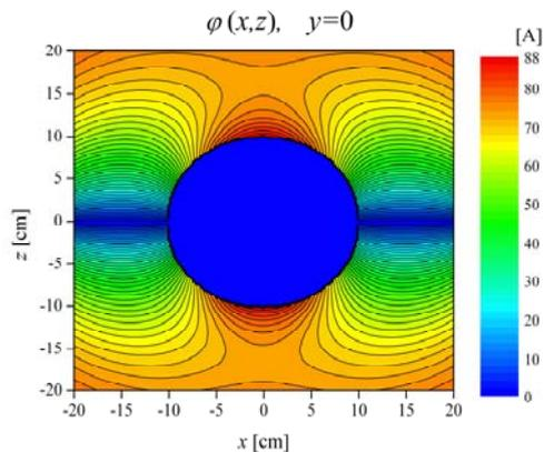
Fig. 6. Computed magnetic potential distribution
