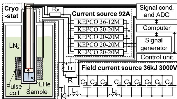
Fig.3. Schematic diagram of the modified Cryo-BI-Pulse system.
