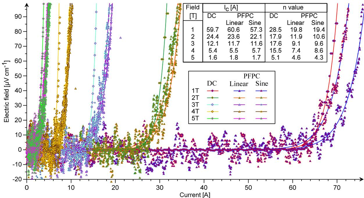
Fig.6 Electric field vs. current recorded from the wire during constant field direct current (CFDC) and pulse field pulse current (PFPC) measurements with two shapes of current ramp (Fig. 2). The inset table presents the critical current  $I_c$  and  $n$  values obtained for each curve.
