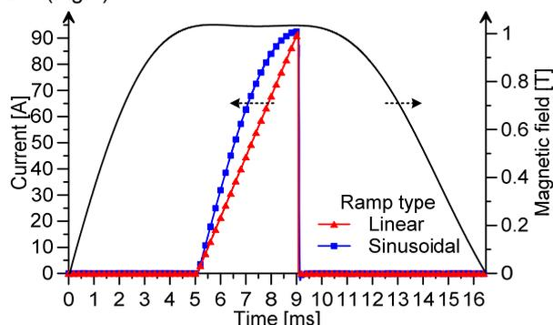
Fig.4. Magnetic field and current pulses used for testing at 4.2 K.
