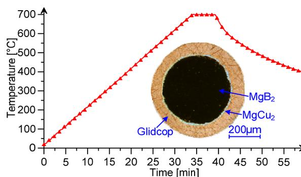
Fig.1 Temperature profiles of the heat treatments of the wire. Insert shows an optical microscope micrograph of the wire cross-section.
