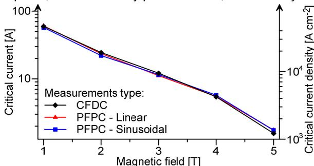
Fig.7. Critical current (density),  $I_c(B)$  ( $J_c(B)$ ), vs. magnetic field from constant field direct current (CFDC) and pulse field pulse current (PFPC) measurements for  $MgB_2$  wire (Fig.1) at 4.2 K.
