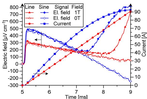
Fig.5 Electric field (left ordinates) signals recorded from the sample during sinusoidal and linear current pulses (right ordinates) without applied magnetic field and during a 1 T magnetic field pulse.
