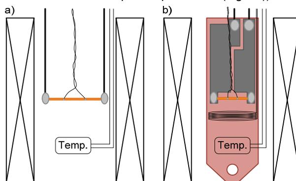
Fig. 2 Schematic diagrams showing the mounting of wire samples for: a) constant field direct current (CFDC) and b) pulse field pulse current (PFPC) measurements. In fig. b), the coil below the sample is used to measure the voltage induced by the pulsed magnetic field, so that this contribution to the sample voltage can be cancelled. Temperature sensors and magnetic field coils are not shown to scale.
