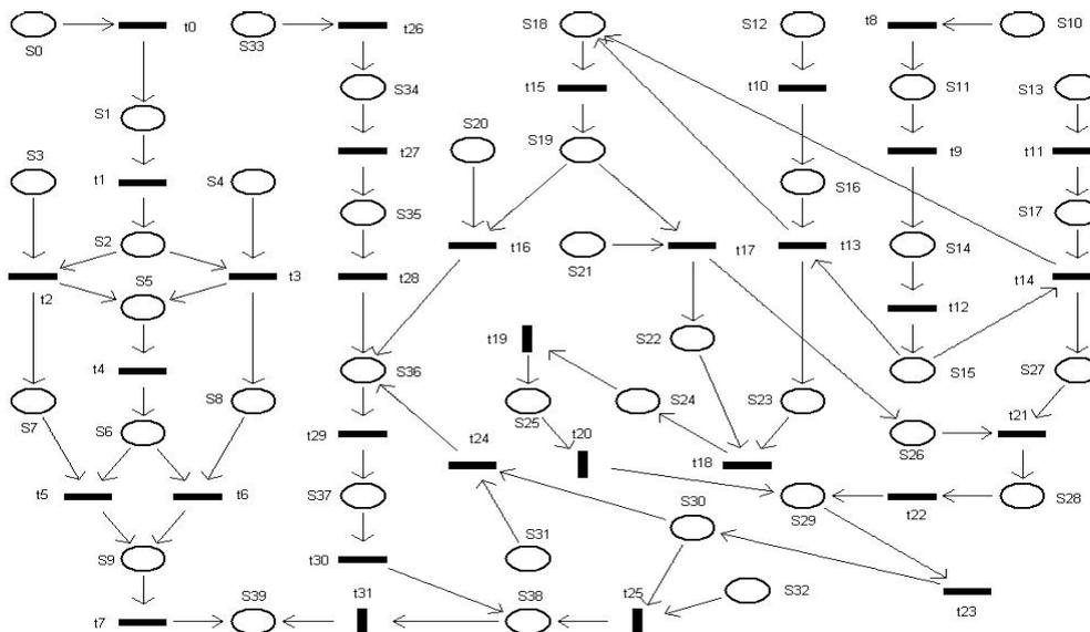
Fig.3. AGSPN model for power transformer fault diagnosis
