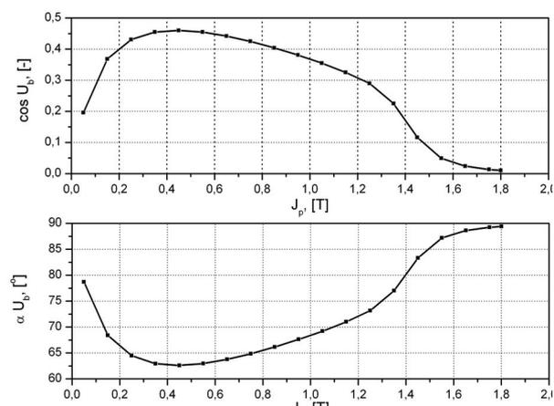
Fig.2. The change of phase shift  $\varphi$  between waveform of measuring voltage and magnetizing current and its cosine (power factor) in function of polarization peak value  $J_p$
