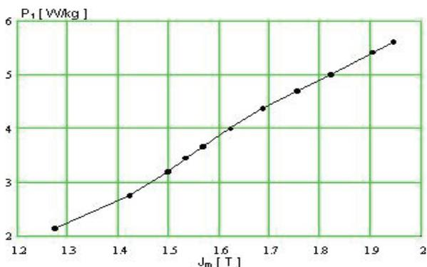
Fig.6. Dependence between loss and peak polarization value
