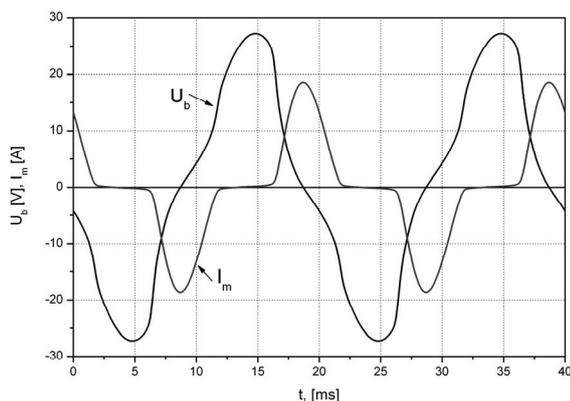
Fig.1. The waveforms of magnetizing current and secondary voltage at high magnetic flux density, instantaneous power ( $H_m = 13\ 800$  A/m,  $J_p = 1.8$ T)
