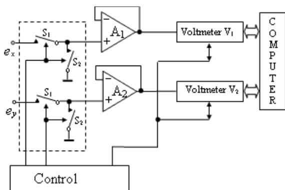
Fig.3. Two-channel system for simultaneous measuring of instant magnetic flux values in coil H (signal  $e_x$ ) and in coil B (signal  $e_y$ ).
