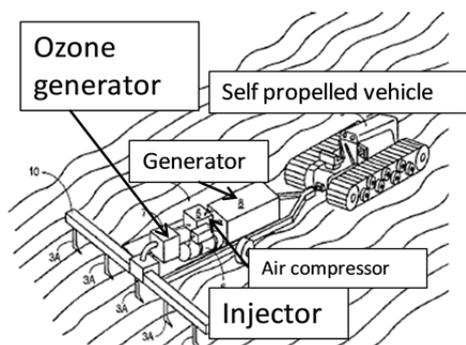
Fig.2. Field sterilization (US Pt. 5624635)
