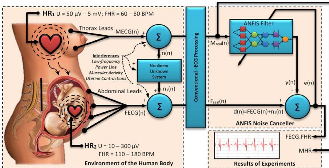
Fig.7. The experimental system designed for FECEG monitoring using ANFIS
